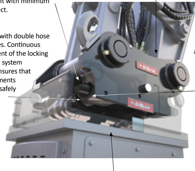
The OilQuick frame has hardened pins, bevelled inner edges, drilled holes for welded pins and enables a precision fit. This ensures connection with no play for minimum wear and long service life.
